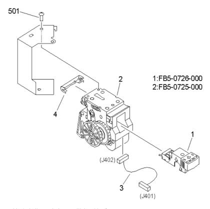
NOTE: This assembly does not include the part shown with key No. 3.
