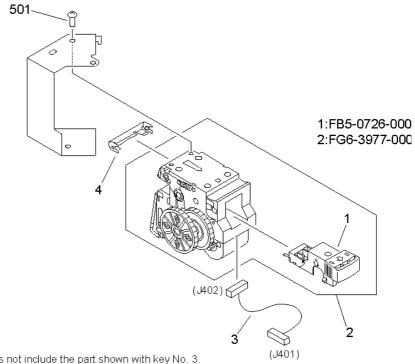
NOTE: This assembly does not include the part shown with key No. 3.
